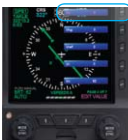
Figure 5-24 Va V-speed Set With New Value
