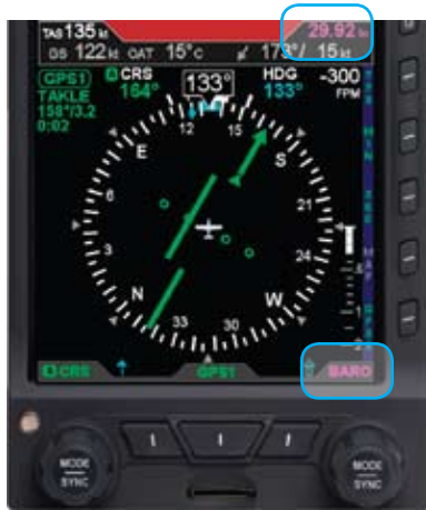
Figure 4-18 BARO Field Enabled
