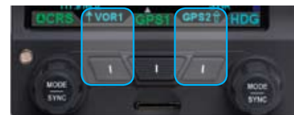
Figure 3-12 Bearing Pointer Nav Source Select Buttons
