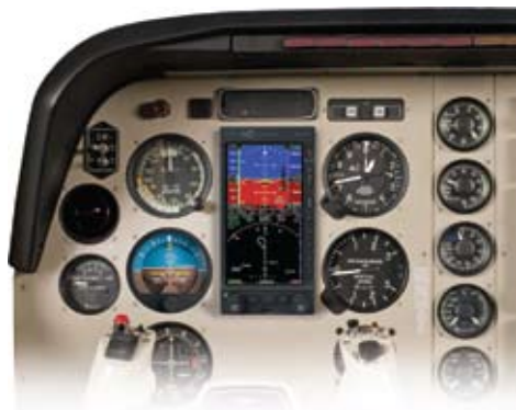
Figure 1-2 Single-tube EFD1000 PFD system
