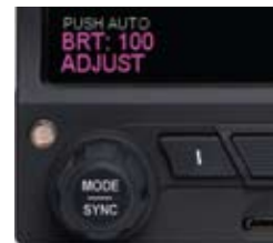
Figure 2-25 Display Brightness in BRT ADJUST Mode
