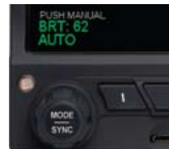
Figure 2-24 Display Brightness in BRT AUTO Mode
