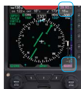
Figure 3-7 BARO Field Enabled
