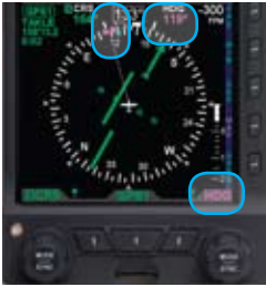
Figure 2-4 Activating the HDG field to edit
