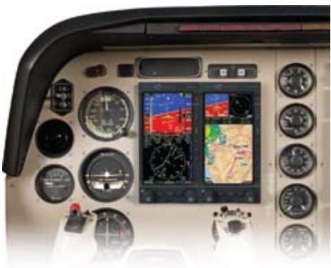
Figure 1-3 Two-tube system: PFD &amp; MFD
