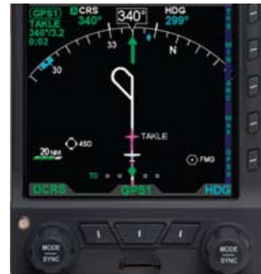
Figure 3-34 ARC Mode Showing Procedure Turn, GPSS Enabled
