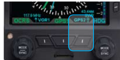
Figure 4-74 Double-Line Bearing Pointer and Button
