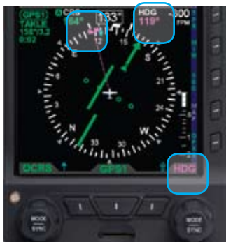
Figure 3-9 Heading Field Enabled
