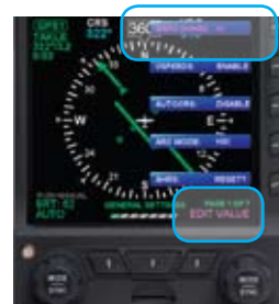
Figure 4-17 BARO Set to mB (millibars)
