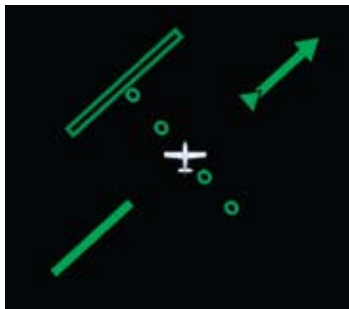
Figure 4-54 Exceeded Deviation, 360° and ARC HSI
