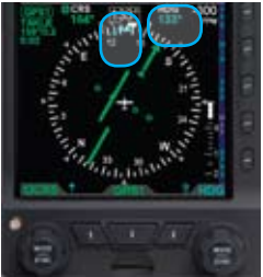
Figure 2-6 HDG field updated and inactive
