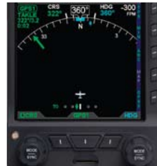
Figure 4-40 ARC Compass Mode
