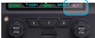
Figure 3-19 Altitude Field Enabled
