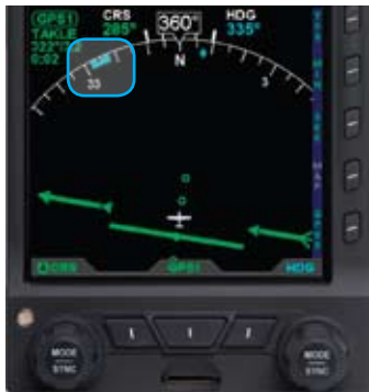
Figure 4-75 Selected Heading Bug and Numerical Display
