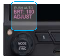
Figure 5-26 Display Brightness in BRT ADJUST Mode
