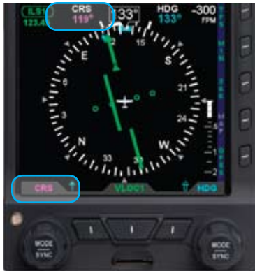
Figure 4-68 CRS Field Enabled for Editing
