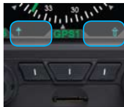
Figure 4-72 Bearing Pointers OFF
