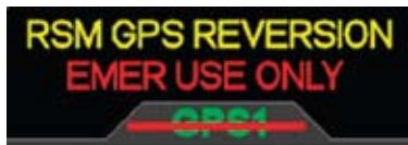
Figure 4-89 GPS1 Failure, Reversionary Navigation
