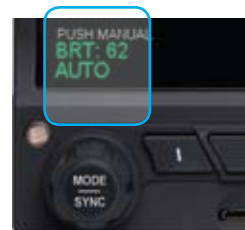
Figure 5-25 Display Brightness in BRT AUTO Mode
