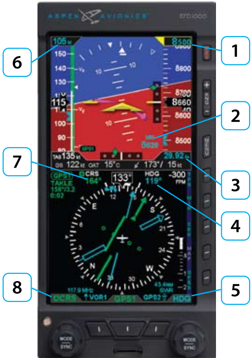
Figure 2-3 Left and Right Knobs and Corresponding Fields
