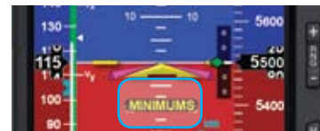
Figure 4-26 Minimums Alert Active
