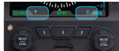
Figure 3-13 No Bearing Pointer Sources Selected
