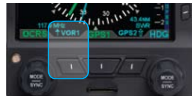
Figure 4-73 173 Single-Line Bearing Pointer and Button
