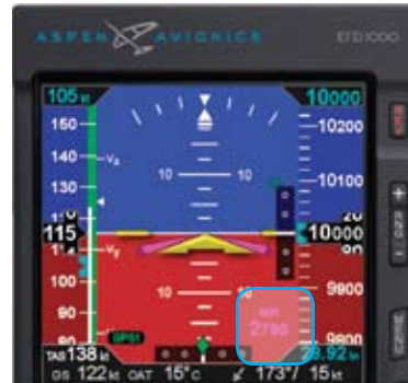
Figure 4-23 Selected Minimums Enabled
