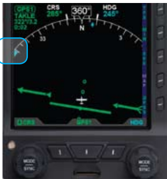
Figure 4-76 Selected Heading Bug Outside of ARC Range
