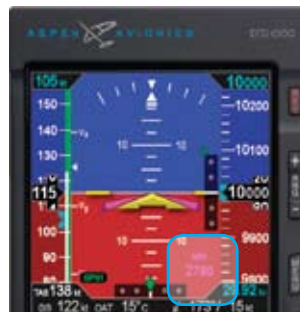
Figure 4-24 MIN Field Enabled
