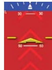
Figure 4-3 Pitch Markings - Large Pitch Up
