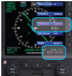
Figure 4-63 AUTO CRS Enabled
