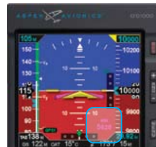
Figure 4-25 New MIN Setting
