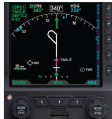
Figure 2-48 Map in ARC Mode, 20nm Range at Feature Level 3 (Medium)
