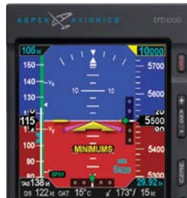
Figure 2-32 Instrument Approach Indications
