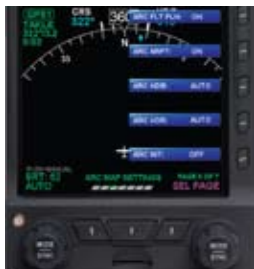
Figure 5-9 ARC Compass Mode Display Options
