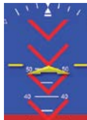
Figure 4-2 Pitch Markings - Large Pitch Down
