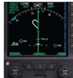
Figure 4-34 ARC HSI Compass Mode
