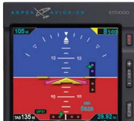
Figure 4-10 Airspeed Tape Disabled
