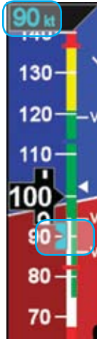
Figure 4-8 New Airspeed Selected
