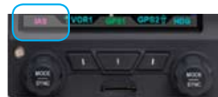
Figure 3-22 Selected Airspeed Bug Enabled
