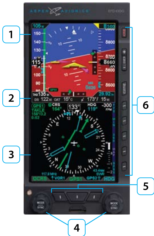
Figure 1 EFD1000 PFD Display, Knobs , Buttons, and Keys
